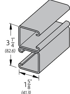
Our welded channels are spot welded 2" (50.8mm) on center, dimensions shown are for welded variations of any channel with or without slotted holes.
