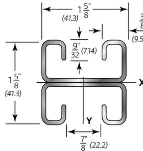
1<sup>5</sup>/<sub>8</sub>" x 1<sup>5</sup>/<sub>8</sub>" (41.3mm x 41.3mm)
